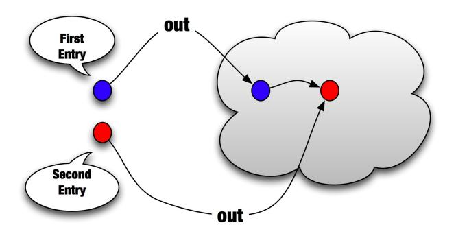
Then an rd operation would return the first entry (the blue one), without removing it from the space. The
