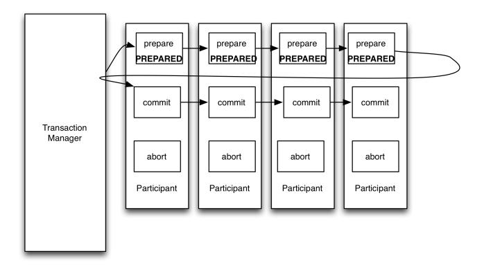
When a participant adds the NO\_JOIN modifier (by returning PREPARED | NO\_JOIN), then the TM skips calling that participant's commit method as shown in the following diagram.
