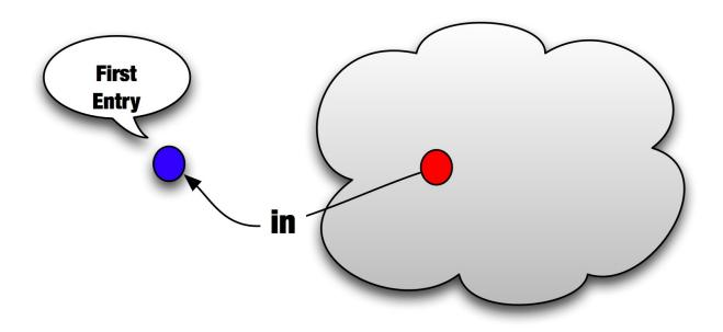
At this point, a new *rd* operation will return the second entry (the red one) and an *in* operation would return the red one as well, leaving the space empty (further *rd* or *in* operations on that particular key will block.
