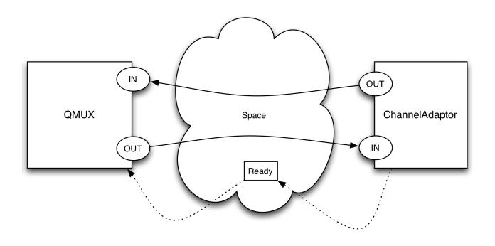
QMUX is registered in the NameRegistrar under the name provided in the qbean configuration file using the "mux." prefix, ("mux.mymux" in our example) so that other components can get a reference, cast it to MUX and use its:
